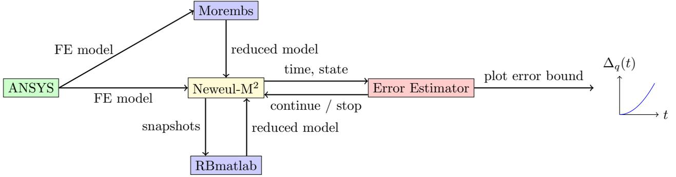
Fig. 3. Involved programs and workflow: The FE model from ANSYS is either reduced directly (based on the system matrices) in Morembs or used in Neweul-M<sup>2</sup> for snapshot generation. These snapshots can then be used in RBmatlab to generate a reduced model. Either way, the reduced model is simulated in Neweul-M<sup>2</sup>. In parallel to the simulation, the error is estimated in a separate Matlab class and used to decide if the simulation should continue or abort.
