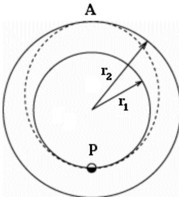
A is the aphelion (point furthest from the Sun) and P is the perihelion (closest to the Sun) of the Hohmann Transfer Orbit. Note that the length of AP is  $(r_1 + r_2)$ .
