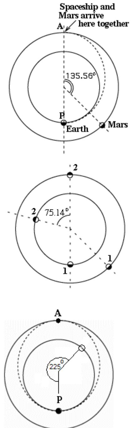
Angle of Mars (relative to 12-o'clock) is  $360^\circ \times (T/1.8822)$ .
